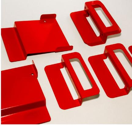
The company is able to change colors in a timely matter since installing its new powder coating system. These brackets for the RV market have been powder coated and are ready to be packaged for delivery.
