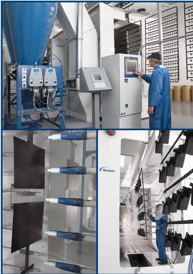
Top: An integrated control system allows for closed-loop digital control of the system and is used in tandem with a PLC-based lean recipe selector (LRS) for automatic selection of spray settings. Bottom Left: Powder is applied using 20 automatic spray guns for precise, repeatable application. Bottom Right: Manual spray platforms on each side of the booth use two manual spray guns for touch up to Faraday cage areas.
